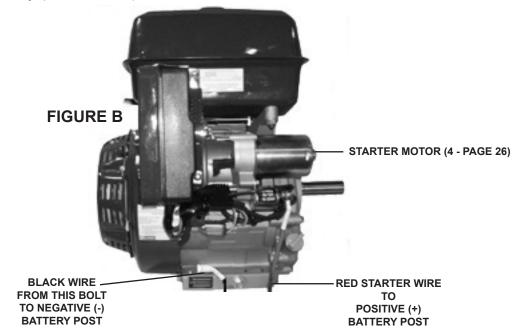
2. To provide battery power to the Starter Motor (4 - page 26), connect the **BLACK** (negative -) wire from the negative (-) post on the battery to the Bolt designated on the base of the engine. Then connect the **RED** (positive +) wire from the Starter Motor to the positive (+) post on the battery. (See Figure B.)
